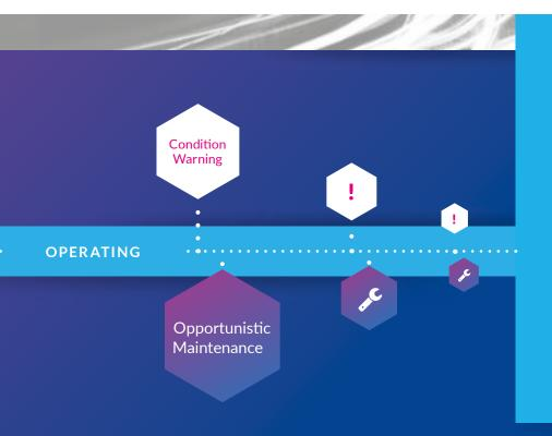
In the context of Industry 4.0, predictive maintenance means using constant, in-situ monitoring of condition indicators, such as vibration and current. These can be monitored inexpensively and easily, with data collection devices connected to the internet. However, analysis still needs to be performed on a mostly manual basis, so continuous CM is often only viable on high-value assets or where a safety case mandates its use.
