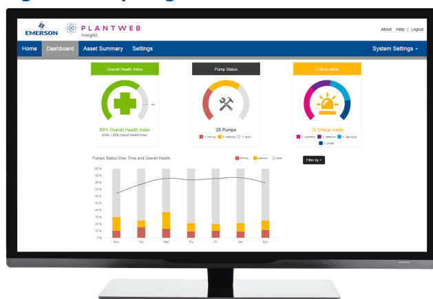
Figure 3. Pump Insight Interface
